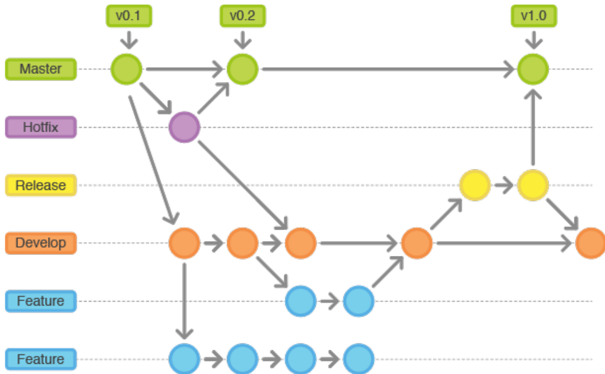
Fig. 7.34: This figure shows typical interactions between branches in the Gitflow workflow. Here, main was merged into develop after tagging version v0.1. A fix was needed and so a hotfix branch was created. When the fix was completed, it was merged into main and develop. Main was tagged with version v0.2. Also, work was performed on two feature branches. When one feature branch was done, it was merged into develop. Then, a release branch was created and it was merged into main when the release was finalized. Finally, main was tagged with version v1.0.
