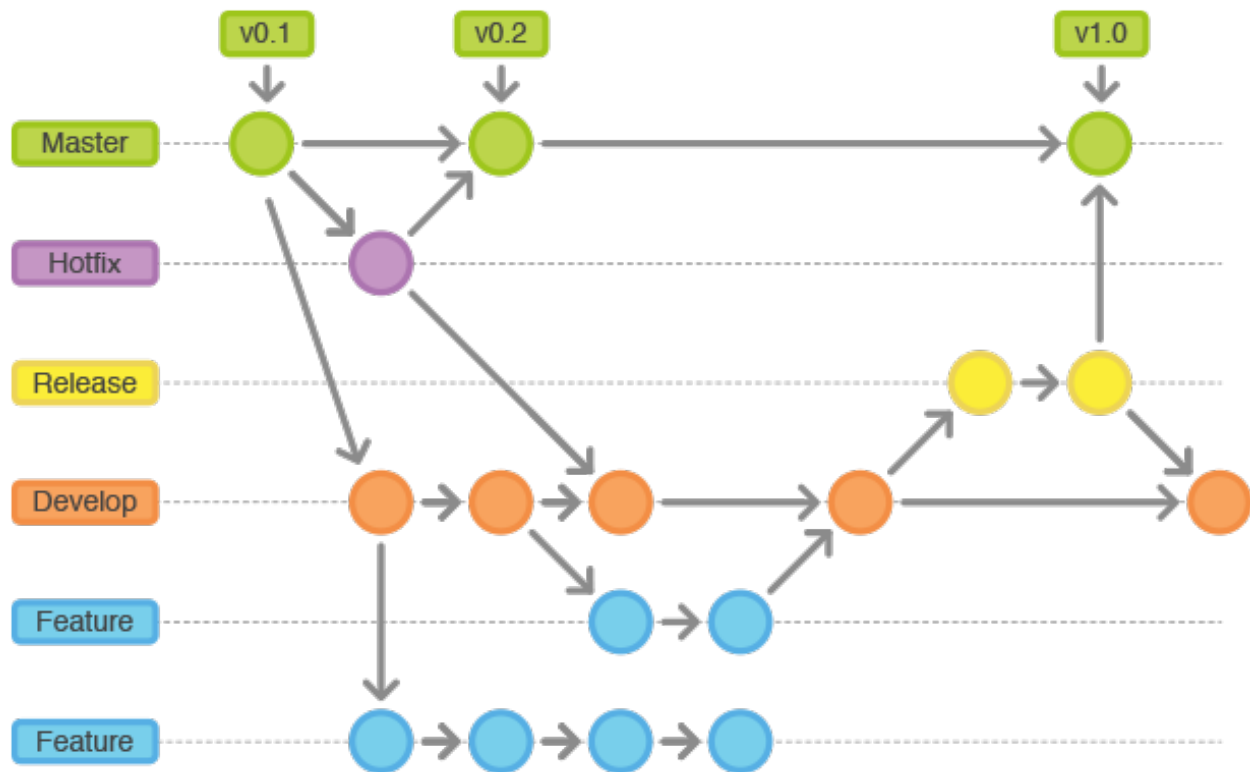
Fig. 3.2: This figure shows typical interactions between branches in the Gitflow workflow. Here, master was merged into develop after tagging version v0.1. A fix was needed and so a hotfix branch was created. When the fix was completed, it was merged into master and develop. Master was tagged with version v0.2. Also, work was performed on two feature branches. When one feature branch was done, it was merged into develop. Then, a release branch was created and it was merged into master when the release was finalized. Finally, master was tagged with version v1.0.
