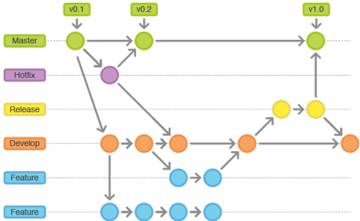
Fig. 7.35: This figure shows typical interactions between branches in the Gitflow workflow. Here, main was merged into develop after tagging version v0.1. A fix was needed and so a hotfix branch was created. When the fix was completed, it was merged into main and develop. Main was tagged with version v0.2. Also, work was performed on two feature branches. When one feature branch was done, it was merged into develop. Then, a release branch was created and it was merged into main when the release was finalized. Finally, main was tagged with version v1.0.
